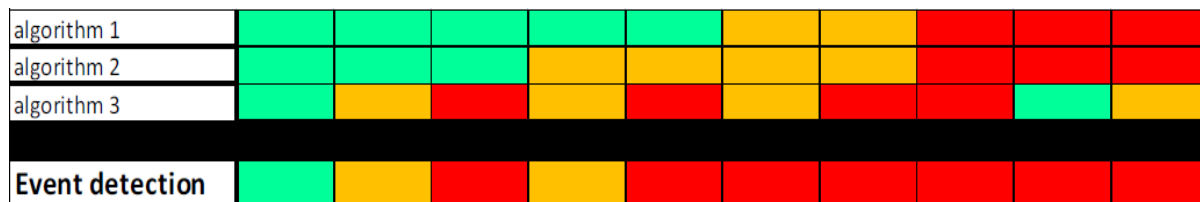
Figure 3: Example of combined event signal logic; ■ Green (OK) ■ Orange (Level 1) ■ Red (Level 2).
